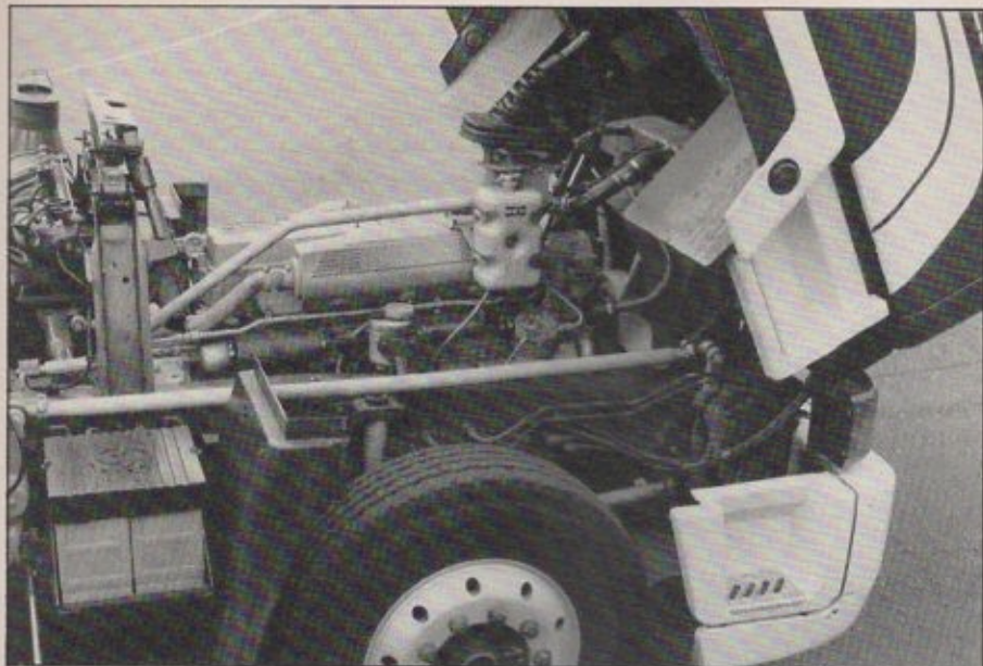
Above: Steering movement to the intermediate axle is via a link-arm running along the outside of the chassis.
