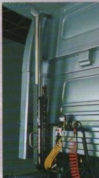
Vertical exhaust and high coupling bridge.
