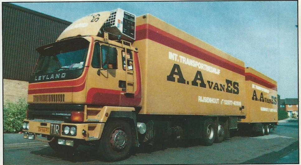
Above: A. AvanES's Rolls Royce 35Ti-powered Roadtrain. Refrigeration is supplied courtesy of Thermo King.
