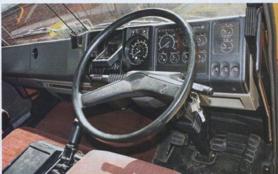
Note the distinctive 'horseshoe' shaped handbrake lever mounted on dashboard.
