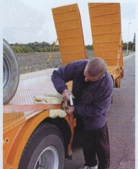
I like how Phil used bits of blanket to protect the paintwork from the tensioner causing damage.
