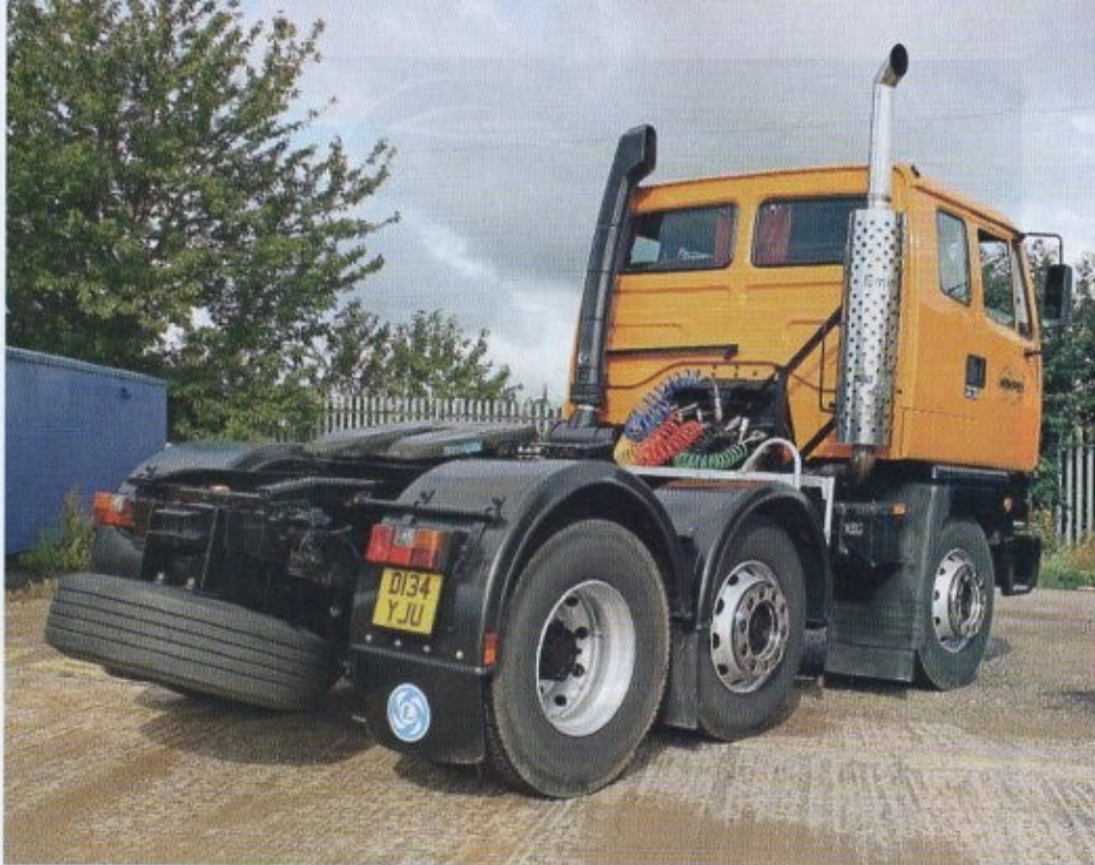
The 6x2 Roadtrain was built so short so that it could legally handle most existing semi-trailers without the need to modify trailer's necks.
