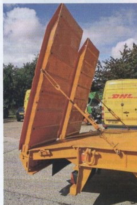
The beaver tail and ramps of the trailer can be removed if required.
