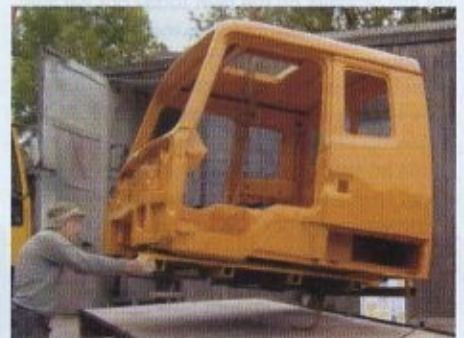
The new cab after spraying being lowered into place by Jack Shinn.
