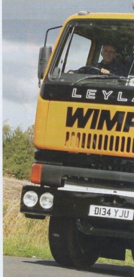
Phil had to have a Roadtrain just like his dad's – with the High Datum cab, a Cummins 320 engine and also with brown carpets and matching brown covered seats.
