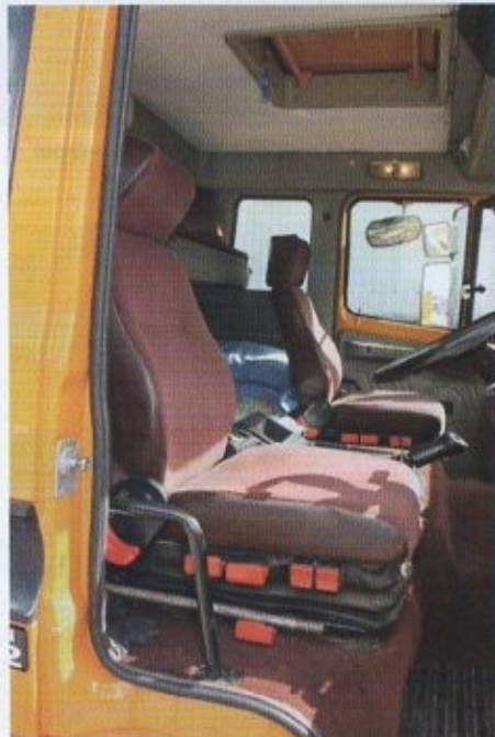
Note the distinctive 'horseshoe' shaped handbrake lever mounted on dashboard.
