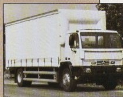
Top: ERF's own factory-built dropframe rigid chassis.
