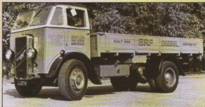
This was the truck that started it all, with its Gardner diesel engine, David Brown gearbox and Kirkstall axles. Leighton Buzzard operator W F Gilbert bought it on 1 September, 1933.
