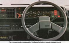
The comprehensive dashboard of the Super includes a graphic display control module, which has an illuminated diagram of the car to pinpoint possible faults, as well as a rev counter and a digital clock.
