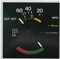
The gear change indicator and econometer. A precise indication of performance efficiency.
