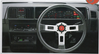
The leather covered three spoked steering wheel and the clear instrumentation of the dashboard. (The radio/cassette is an optional extra.)
