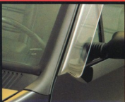
Anti-turbo baffle integral with covered upright.
