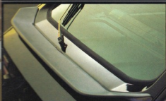
Rear spoiler — an eye-catching feature which significantly improves drag.
