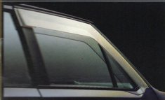
New front door anti-turbo baffles. This innovation alone allows maximum speed to be increased by 2.8 kph.
